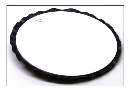
The sampling plate is 10.5" (27 cm) in diameter, and provides a large sampling surface for conditions saturated to 50 cb. of suction. It has a butyl rubber backing and uses a stainless steel tie wire, and a stainless steel sampler outflow stem on the bottom side of the sampling plate.
