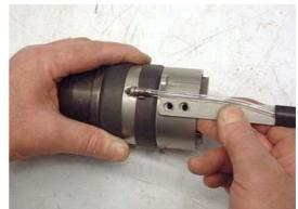
Place the crosspiece of the clamping tool in position and fit the ring and swivel. Make sure all the parts are properly centred and check this when tightening the swivel.
