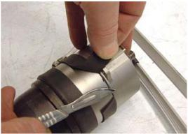
Push the ring with clamping pins over the cutting ring and fit the new nuts that are included in the set by hand. Tighten the nuts **alternately and a little further each time** using the box spanner. After that, you can remove the clamping tool and fit the cutting head back into the frame.
