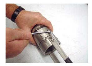
Take the cutting head and the small box spanner from the tool set. Remove the three nuts from the cutting head by loosening all three slightly first and then unscrewing them further. Remove the ring with the threaded pins, the upper collar, the cutting ring and the damaged membrane.
